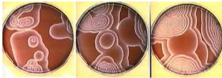
Figure 2.1 Pattern formation in the Belousov-Zhabotinskiy reaction [20].
