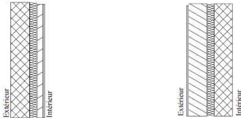
Figure 5: isolation entre murs
