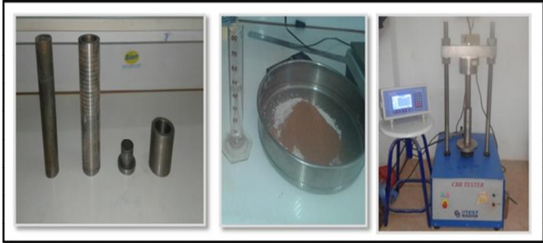
Photo III.1: Essai de compactage statique
